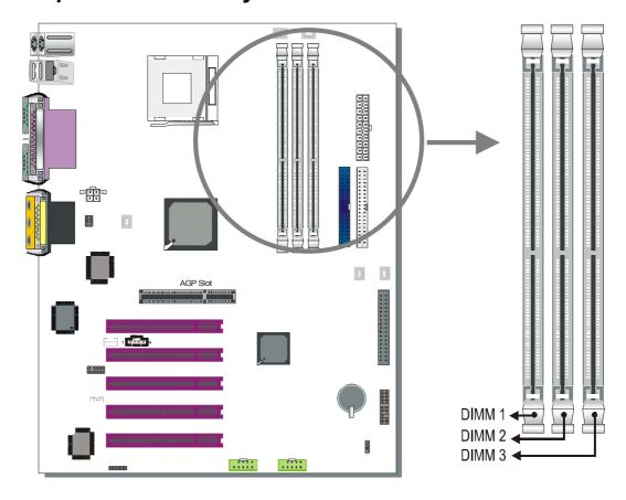
Your board comes with three DIMM sockets, providing support for up to 3GB of main memory using unbuffered and non-ECC DIMM modules from 64MB to 1GB. On this motherboard, DRAM speed can be set independent from the CPU front side bus speed. Depending on the DRAM clock speed setting in the BIOS setup, appropriate memory modules must be used. For 100MHz DRAM speed, use PC1600 memory; for 133MHz DRAM speed, use PC2100 memory; for 166MHz DRAM speed, use PC2700 memory.
